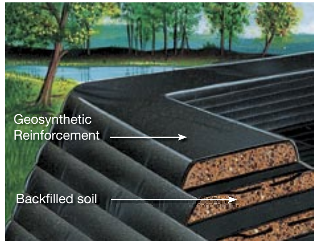
Internally reinforced earthwall
